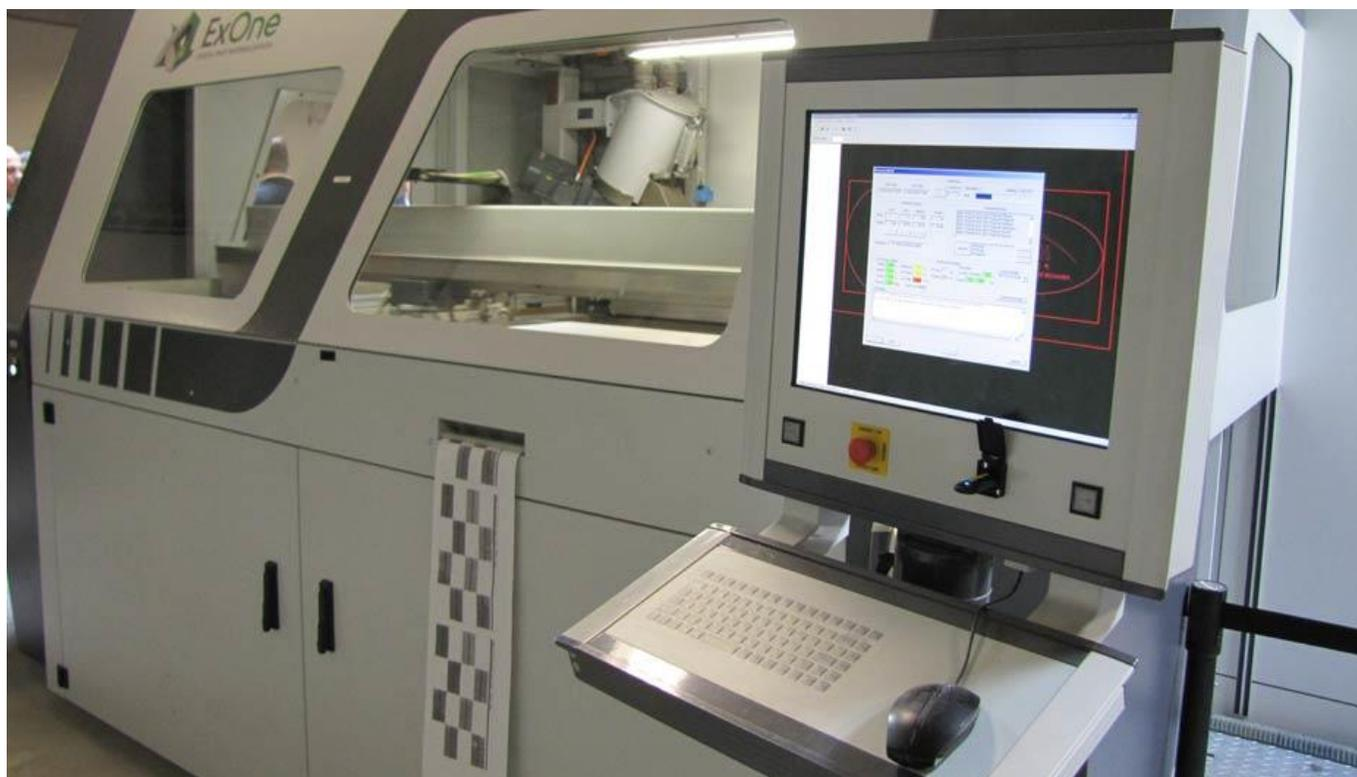
It is the only printer of its kind in the state, and Conner said there is room in the building for one more. “This is a very large printer,” he said, noting the build parameters measure six feet in length, three feet in width and about two feet in depth. “Technologies like this are used to make prototype engine components, such as an engine block for an automobile.”
