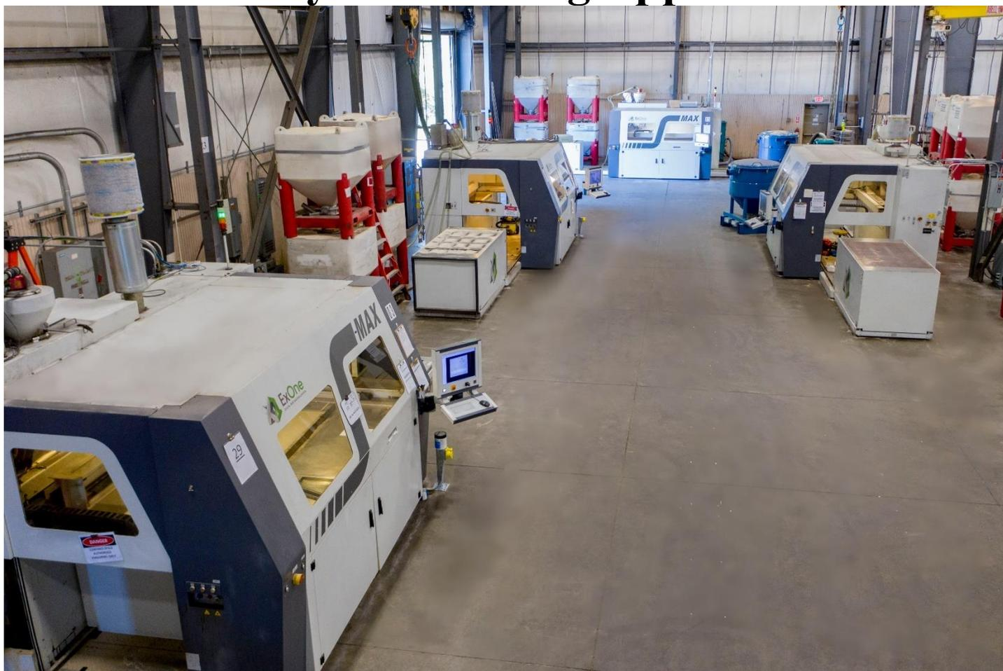
The foundry industry is one of the oldest trades known to mankind, and until recently has been practiced very much the same way as it has been for centuries. Additive Manufacturing has brought disruptive innovation to this industry. Traditionally, the metal casting process involves creating a tool or pattern to create the sand core and mold. However, with Additive Manufacturing, you can directly print the sand core and mold through software commands without any tooling.
