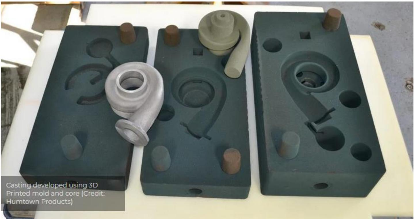
To summarise, the applications which are very suitable for AM are pumps, impellers, complex valve body or complex casting housings for turbos in the automotive industry.
