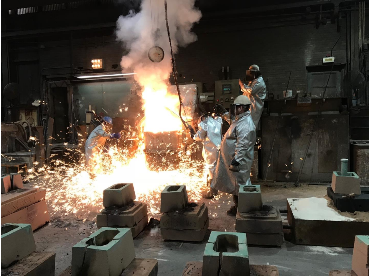
Fig 1. Example of a 2500 kg (5500 lb.) Pelton injector being poured in a multi-part 3D sand printed mold Credit: Kirk Rogers .
