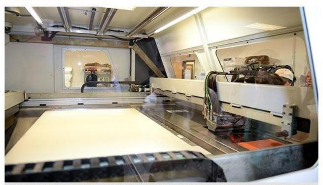
The ExOne S-Max has a 1,800x1,000x700-mm / 70.9x30.4x27.6-in. build area (LxWxH), with a build speed of 2.12-3.00 ft<sup>3</sup>/hour. Joel Lewis, YSU
