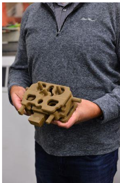
A 3-D printed sand mold used to cast a complex metal part. Photo: Humtown Additive
