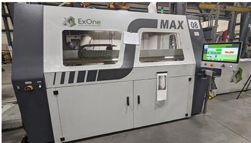
3D printers have transformed Humtown's sand core manufacturing business.
